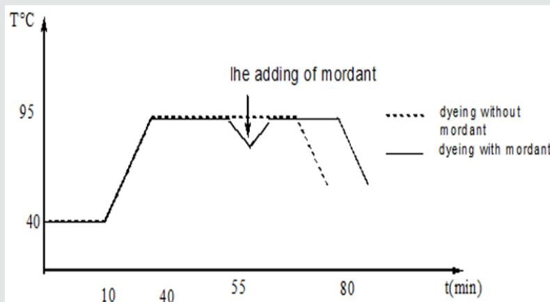
Figure 1: Dyeing process of wool fabric.
