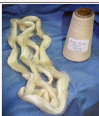
PALF fibre and blended yarn in Eri Spinning system
