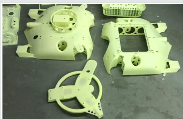
Figure 24: The underwater robot module parts after 3D printing is completed.
