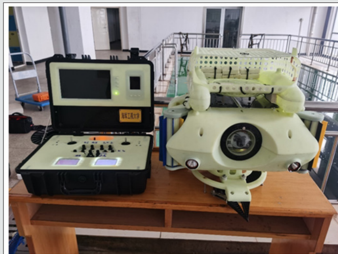
Figure 26: Terminal control box and underwater robot prototype.
