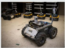
**Figure 1:** Illustrates a small unmanned Clear path Husky robot, which was used by ARL researchers to develop a new technique to quickly teach robots novel traversal behaviors with minimal human oversight. Image Credit: US Army [2].
