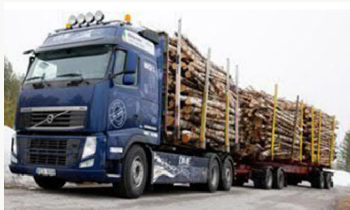
Figure 3: VOLVO heavy truck running on Dimethyl ether.
