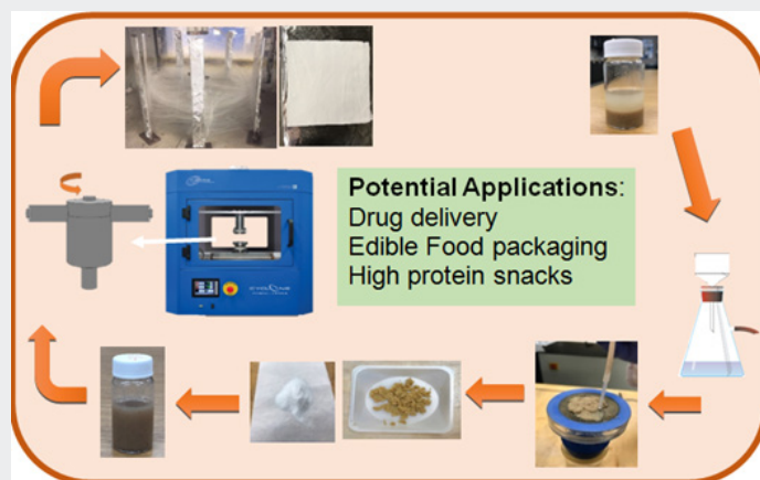
Figure 1: A solution of GCSM and pullulan was prepared and further used to develop fine fibers using the Forcespinning® process. From top right corner, clockwise. The process begins with the GCSM aqueous solution which, is placed under vacuum filtration to remove water. The GCSM and pullulan powders are then weighted, and desired concentrations placed in an aqueous solution. This solution is then spun using the Cyclone L-1000M which uses a two-nozzle spinneret. The developed fibers are then collected in 4"×4" mats.
